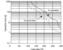
(10)Over-temperature protection for motor
