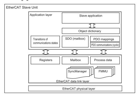
The objects in the object dictionary for the CAN application protocol are broadly divided into PDOs (process data objects) and SDOs (service data objects).
