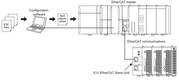
Communications are started according to the communications settings and the network configuration in the ESI files that are installed.
