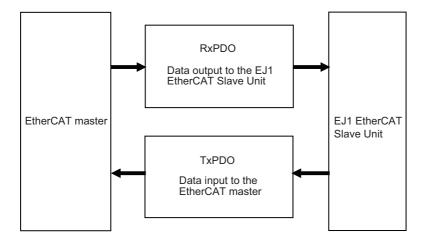
The EtherCAT application layer can hold more than one object to enable the transfer of various process data of the EJ1 EtherCAT Slave Unit.
