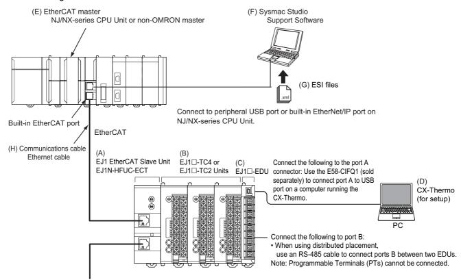
A maximum of 15 Basic Units can be connected side by side next to an EJ1 EtherCAT Slave Unit to perform EtherCAT communications through the EJ1 EtherCAT Slave Unit.
