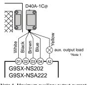
Note 1. Maximum auxiliary output current is 10mA.
