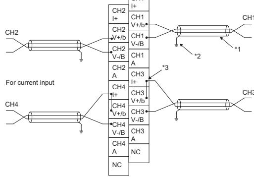
\*1 For the wire, use the 2-core shielded twisted pair cable.
