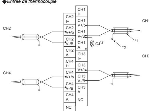
\*1 Always use the shielded compensation lead wire for the cable.
