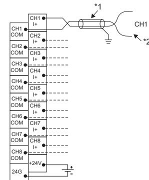
\*1 For the wire, use the shielded twisted pair cable.
