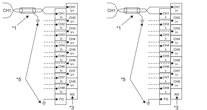
\*1 For the wire, use the shielded twisted pair cable.
