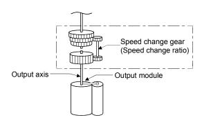
(2) When a speed change ratio changes, the acceleration/deceleration processing is executed by the smoothing time constant (t) set in the speed change gear parameters.
