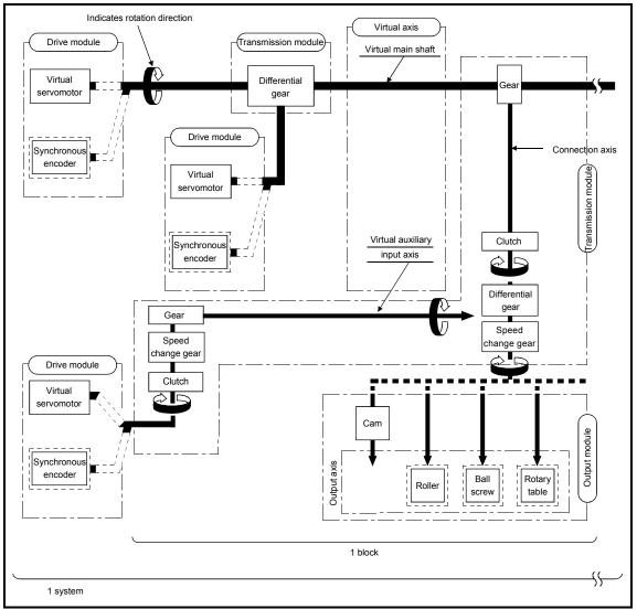
Fig. 5.1 Configuration of the Mechanical Module Connection
