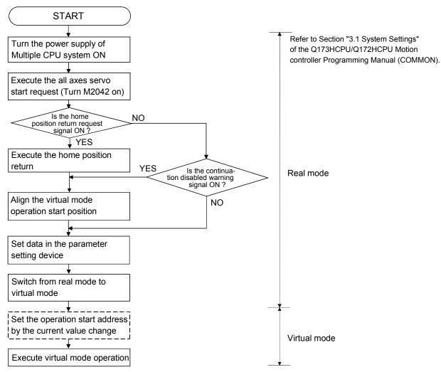
The operation procedure for absolute system is shown below.
