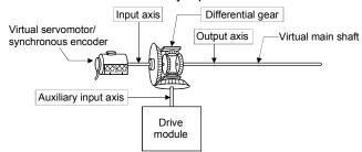
Set the different drive modules for virtual main shaft side and auxiliary input axis side.
