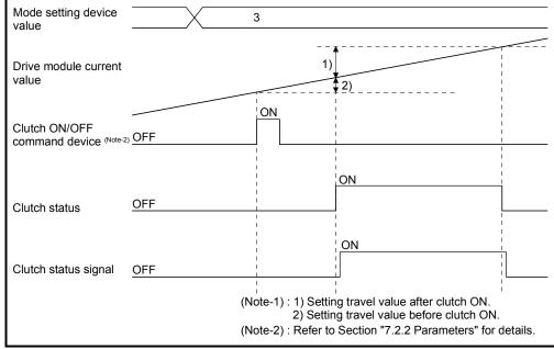
Fig. 7.5 Operation Timing for One-shot Mode
