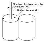
(b) The roller cycle speed is calculated by the roller diameter and number of pulses per roller revolution as the formula below.
