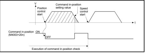
Fig. 6.1 Command in-position range
