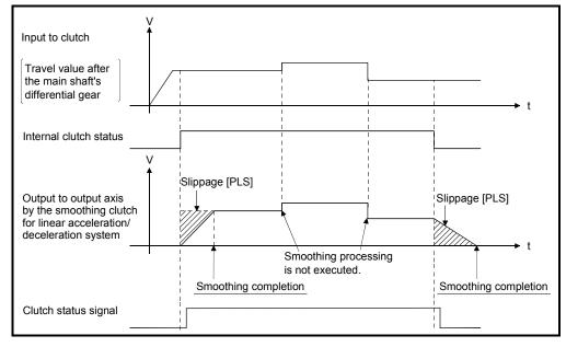
d) If input to clutch (travel value after the main shaft's differential gear) changes after smoothing completion, the smoothing processing is not executed and output directly.
