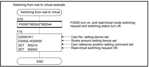
(Note) : Example of the above Motion SFC program is started using the automatic start or PLC program.
