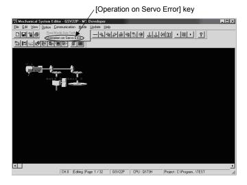
· Operation setting screen on servo error
