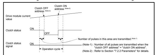
2) When the clutch status signal is ON and the current value passes through an address set in the clutch ON/OFF address setting device.
