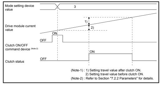
(g) When the mode setting device becomes "3", the clutch status turns OFF, while the clutch ON/OFF command device is OFF and the clutch status is ON.
