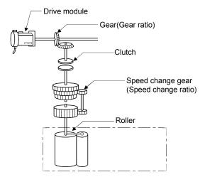
(b) When a clutch is used, the roller is controlled at clutch ON.
