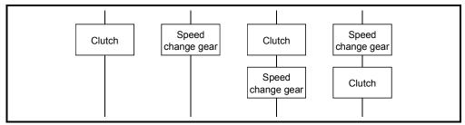
(b) Transmission module which can be connected at "C" (pattern 3) Only a clutch can be connected at "C".
