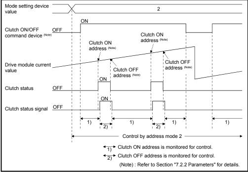
Fig. 7.4 Operation Timing for Address Mode 2
