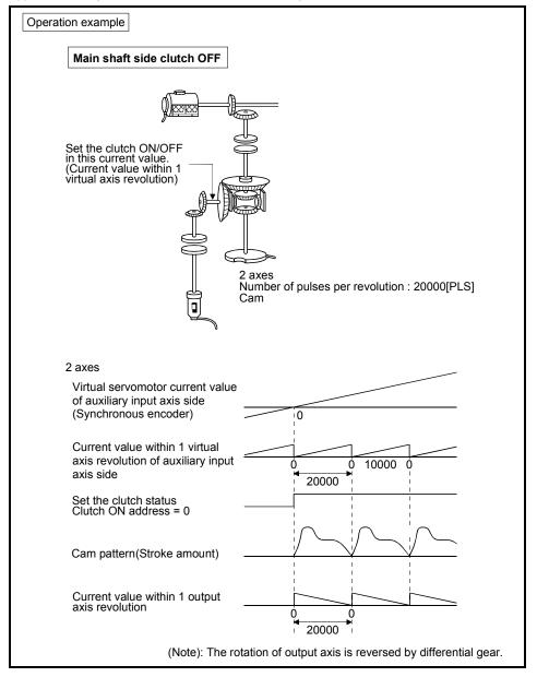
(f) An example of an address mode clutch operation is shown below.
