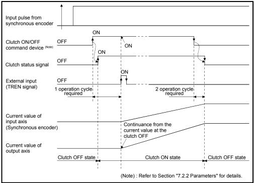
(d) The current value of input axis (synchronous encoder) changes at the clutch ON state only.
