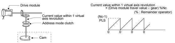
(a) The current value within 1 virtual axis revolution of cam main shaft side is stored in the preset device.
