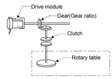
(b) When a clutch is used, the rotary table is controlled at clutch ON.
