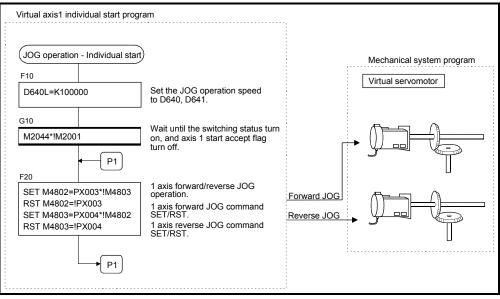
(Note) : Example of the above Motion SFC program is started using the automatic start or PLC program.
