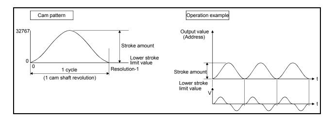
2) Feed cam mode ......With the lower stroke limit value (lower dead point) as the operation start position, positioning is executed by feeding one stroke
