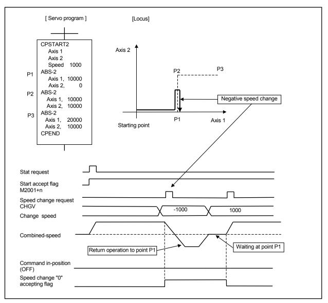
If a speed change to a negative speed is made during execution of positioning to P2 as shown above, the axis returns to P1 along the program specified locus and waits at P1.
