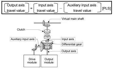
(b) When the input axis clutch turned off.
