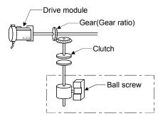
(b) When a clutch is used, the ball screw is controlled at clutch ON.
