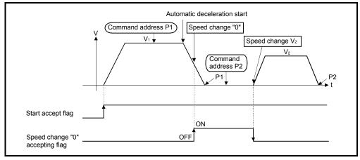
(d) Even if it is speed change "0" after the automatic deceleration start to the "command address", speed change "0" accepting flag turns on.
