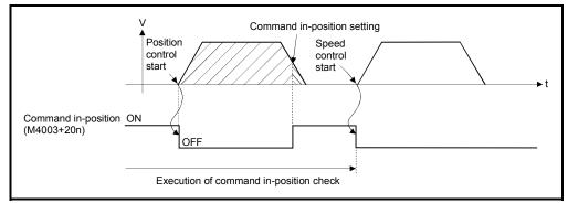
(b) Command in-position check is continually executed during position control. This check is not executed during speed control.
