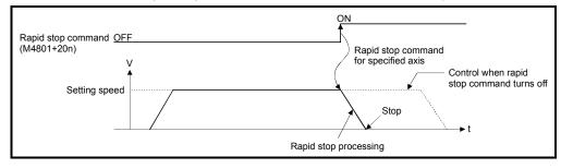
(b) The details of stop processing when the rapid stop command turns on are shown in Table 4.2.
