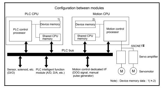
Fig.4.1 Flow of the internal signals/external signals
