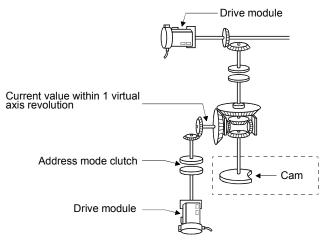
(a) By setting the current value within 1 virtual axis revolution of auxiliary input axis side, for the current value within 1 virtual axis revolution is stored in the preset device.
