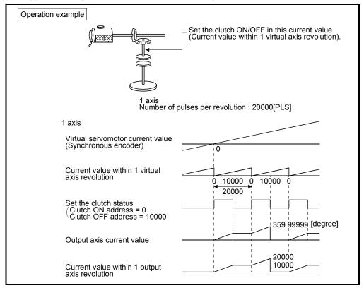
(f) An example of an address mode clutch operation is shown below.
