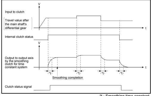
2) If input to clutch (travel value after the main shaft's differential gear) changes after smoothing completion, the smoothing processing is executed at that point.
