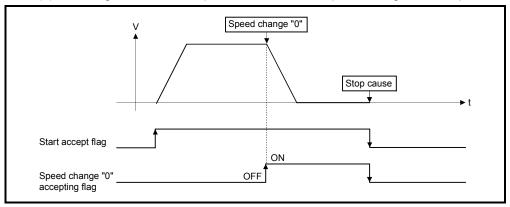
(c) The speed change "0" accepting flag does not turn on if a speed change "0" occurs after an automatic deceleration start.
