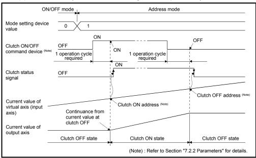
(e) The refresh cycle of clutch status signal is an operation cycle.
