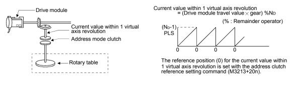
(a) The current value within 1 virtual axis revolution of rotary table main shaft side is stored in the preset device.
