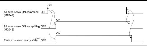
(Note): Refer to Section "3.1.1 Axis statuses "Servo ready signal"" of the Q173CHPU/Q172HCPU Motion controller (SV13/SV22) Programming Manual (REAL MODE) for details.
