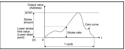
(b) The cam data table is automatically created by creating the cam curve using a peripheral device.
