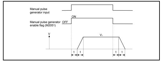
Output speed (V<sub>1</sub>) [PLS/s] = (Number of input pulses/s) × (Manual pulse generator 1-pulse input magnification setting)
