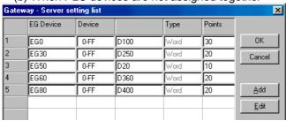
When 100 points of devices are accessed, access to the PLC must be made five times.
