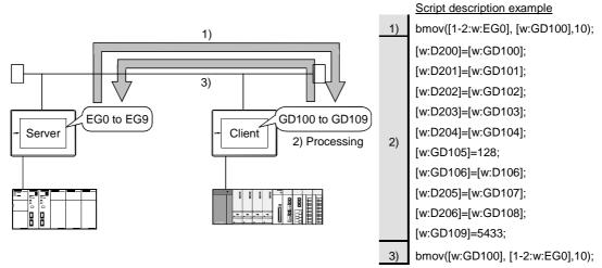
(2) When using gateway devices directly Access to the other station GOT occurs 10 times (1) to 10)). When one time of access requires 50ms, the necessary processing time is about 500ms.
