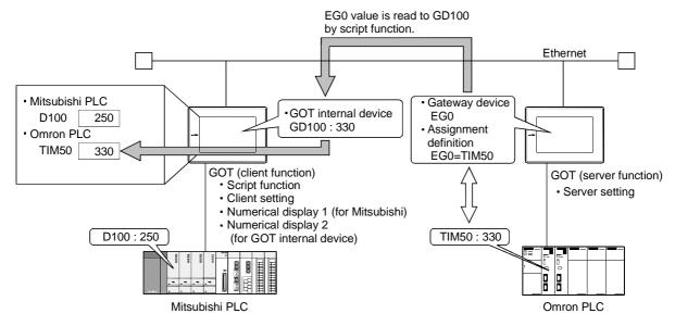
\*The read destination of the script function can be set to the device of the Mitsubishi Electric PLC.
