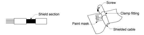
Note) The method of earthing by soldering a wire onto the shield section of the shielded cable as shown below is not recommended. The high frequency impedance will increase and the shield will be ineffective.
