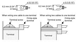
Tighten the terminal screws (M3 screws) on the terminal block with a tightening torgue of 42 to 58 N · cm.
