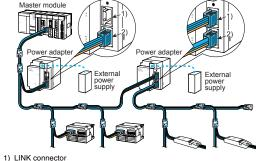
\*1 Some remote I/O modules for CC-Link/LT supply the power for I/O via the flat cable dedicated to CC-Link/LT. For the details, refer to the instruction manual of each remote I/O module.
