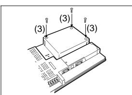
(3) Tighten and fix the mounting screws (3 pcs.) of the A9GT-BUS2SU in the specified torque range.
