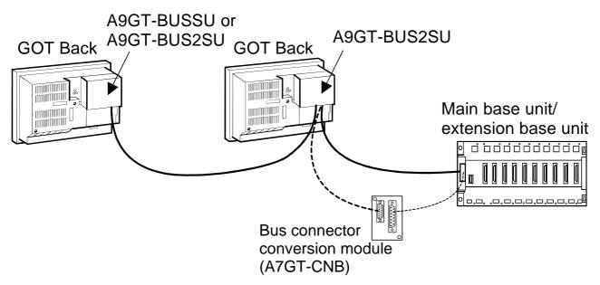
With the A9GT-BUS2SU, the dimensions of the cable that protrudes from the bottom of the GOT are smaller than the A9GT-BUSS/A9GT-BUS2S type bus connection interface board (hereinafter, bus connection board) used with the conventional bus connection.
