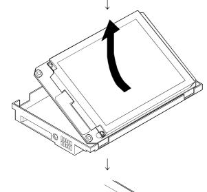
Remove the liquid crystal display and circuit board from the rear case by holding up the top side.
