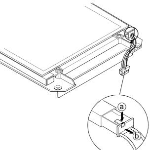
Pull out the backlight in **(b)** direction pressing the fixing tab (black) in **(a)** direction.
