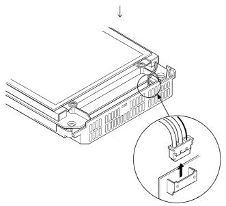
Remove the cable connector for backlight.
