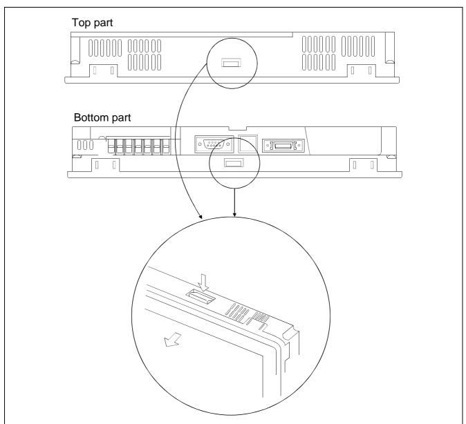
4) After removing the fastening screws, remove the indicator cover from GOT, while pressing two fastening hooks.
