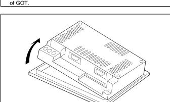
4) Remove the display unit cover on the back of the GOT.
