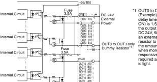
\*1 OUT0 to OUT3 only (Example) The output delay time (OFF to ON) is 1.5 us where the output current is DC 24V. 50mA, Install an external dummy resistor to increase the amount of current when more responsiveness is required and the load
