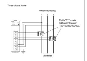
Three-phase 3-wire (with the voltage transformer for gauge/current transformer)
