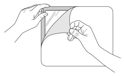
4) Install the Protective Cover on front of Display.
