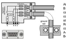
At least data lines A and B (pins 8 and 3) and the cable shield must be connected at each station.
