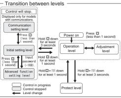
Transition to Communication setting level Press the  $[\Box]$  key for at least three seconds to move from the operation level to the initial setting level; press the  $[\Box]$  key once again to move to the communication setting level.
