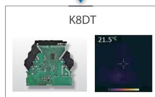
The K8DT-series Relays, however, use a switch mode power supply. There is no heat resulting from inverter noise, for safe, reliable application.
