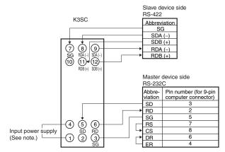
Note: Either a 100 to 240-VAC or 24-VAC/VDC (no polarity) input power supply is used.
