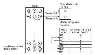
Note: 1. If RS-485 is selected as the communications method (i.e., pin 9 of the DIP switch is set to OFF), terminals 8 and 9, and terminals 11 and 12 are connected internally.
