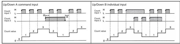
H: Short-circuit ON-time impedance; 1 k $\Omega$  max. Residual voltage; 0.5 V max.
