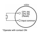
\* Make sure that the contact can switch 0.5 mA at 5 V with ease.
