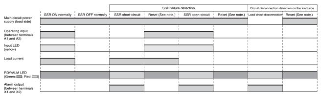
Note: After failure detection, if the detection conditions differ to the conditions given under Conditions for SSR Failure Detection, alarm output is reset.
