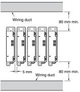
Note: Use the G3PC at a load current of 80% of the rated load current when it is mounted side by side.
