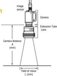
Note: Extension tube length should not exceed 10% of the focal length of the lens. When looking at other manufacturer's lenses, please remember the F150 has a 1/3-inch CCD.
