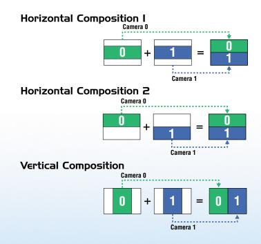
In applications requiring higher-speed inspections, or with a smaller inspection area, operators can configure the controller to process and combine images from both cameras simultaneously.
