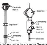
Note: When using two or more Separators, be careful with the mounting direction of the connecting nut screws which connect electrodes. Avoid the screws from touching each other.
