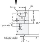
Robot cable of 2.8 dia., 4 cores, (0.15 mm² with 0.8 mm dia. insulator); Standard length: 1 m
