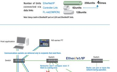
Star topology using Ethernet switch technology
